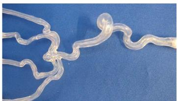
ELASTRAT in vitro models respect human anatomy and are designed for the development and demonstration of stents, coils and catheters. They provide a realistic environment for the simulation of endovascular procedures, pre-surgery training, studies and teaching purposes for interventionists.
