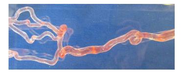
ELASTRAT in vitro models respect human anatomy and are designed for the development and demonstration of stents, coïls and catheters. They provide a realistic environment for the simulation of endovascular procedures, pre-surgery training, studies and teaching purposes for interventionists.
