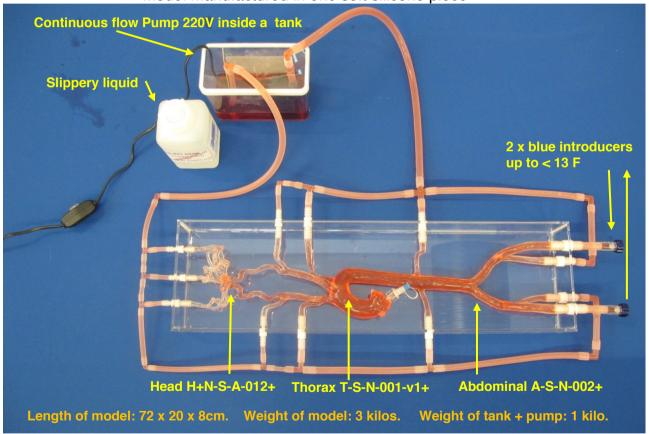
Pump characteristics: Compact continuous flow pump 170-300 l/h, 7 W, 220 - 240 V / 50 Hz
