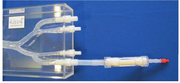
Example of a neuro "Specific Patient" model with connector ID 4mm or 6mm
