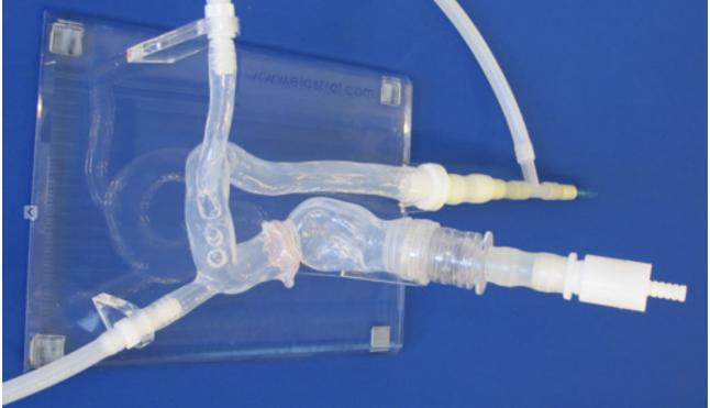
ELASTRAT in vitro models respect human anatomy and are designed for the development and demonstration of stents, coïls and catheters. They provide a realistic environment for the simulation of endovascular procedures, pre-surgery training, studies and teaching purposes for interventionists.
