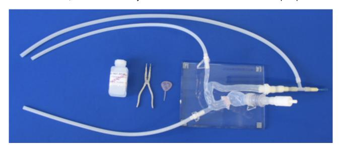
This model contains the aortic arch, the left ventricle and an exchangeable aortic valve
