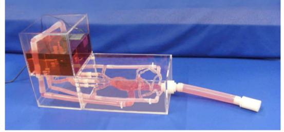
ELASTRAT in vitro models respect human anatomy and are designed for the development and demonstration of stents, coïls and catheters. They provide a realistic environment for the simulation of endovascular procedures, presurgery training, studies and teaching purposes for interventionists.
