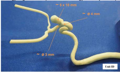
Soft silicone model inside its Plexiglas support, ED of plexiglas support: 180mm L x 100mm W x 90mm H
