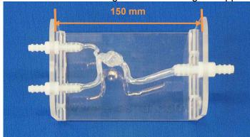
Head model shown with a plastic tank of 2 liter and a continuous flow aquarium pump
