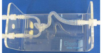
Head model shown with a 1 liter plastic tank and a continuous flow pump
